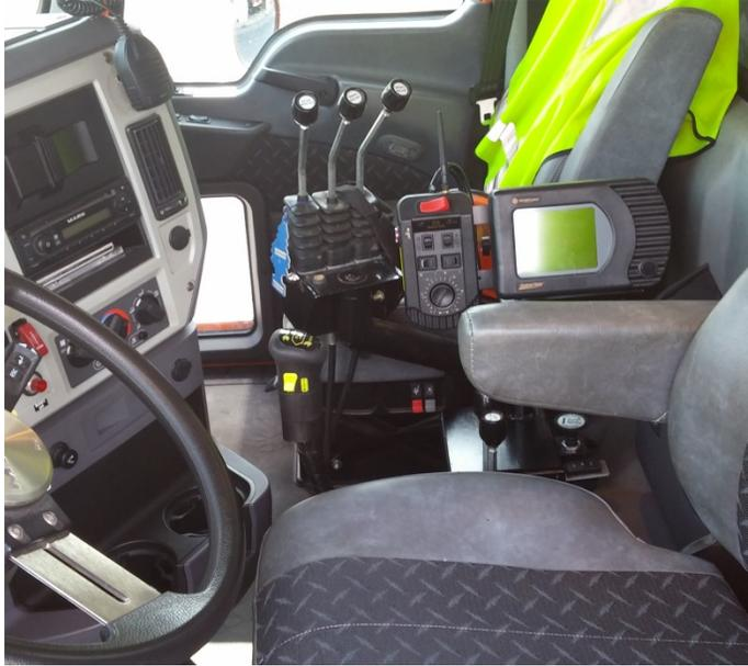
The Dickey-john equipment is installed at the right hand of the Town of Lake George plow truck driver.
